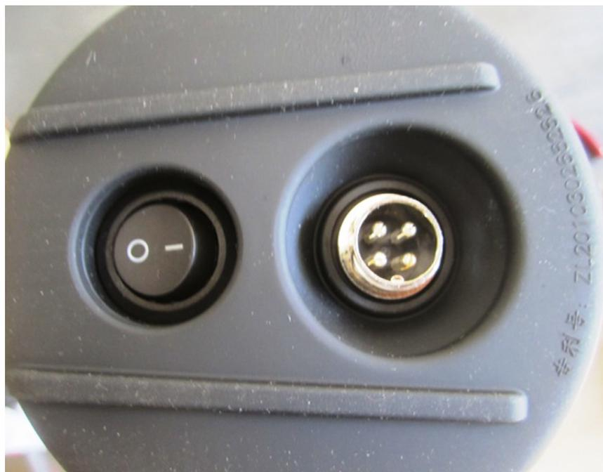
2. Turn power on. Depress On Button until it lights up. – (straight line) is on.
